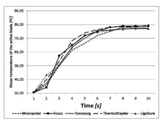
Figure 1. Mean temperature of active blade of investigated devices during prolonged use
